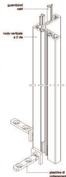
Nodo variabile (da 180° a 85°) Variable corner connector (from 180° to 85°)
